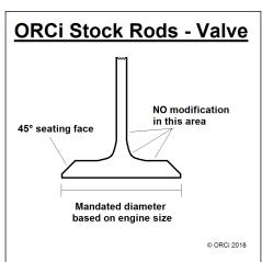
MUST remain as per the manufacturer's original specification. Any other modification to the valve head, stem or profile is NOT permitted. See illustration for reference.
